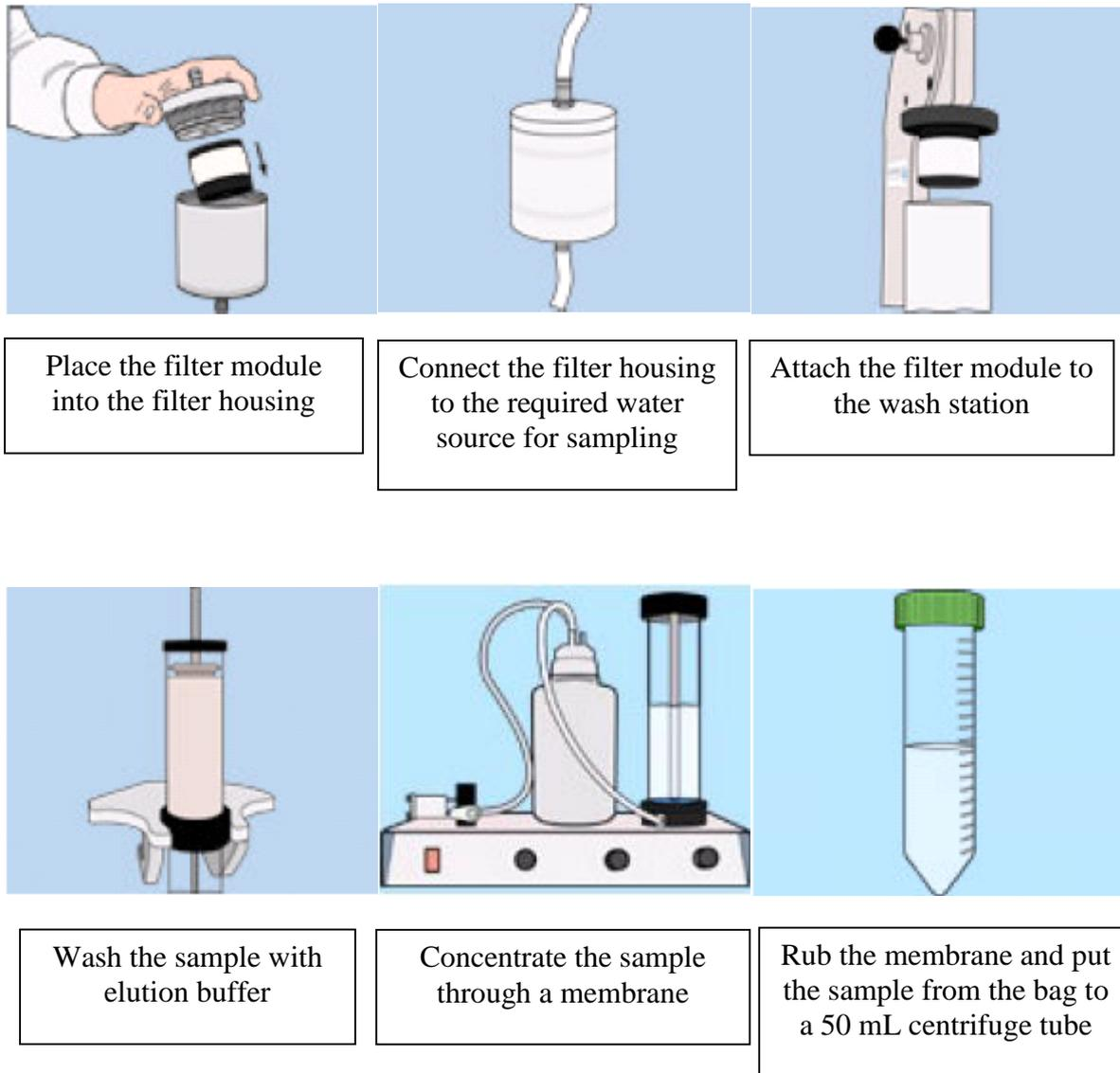
*Figure 2: Schematic representation of the elution protocol*
