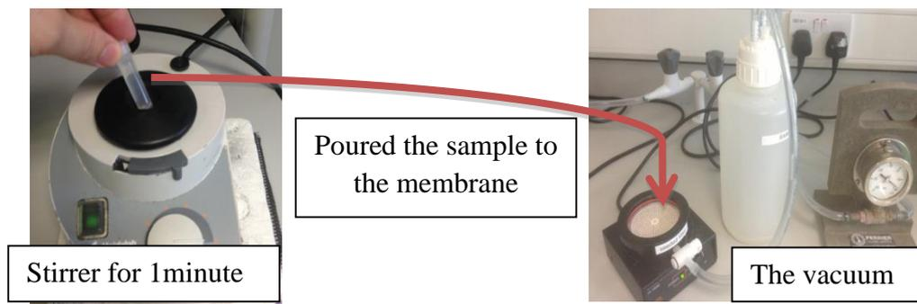
Figure 4: The membrane test
