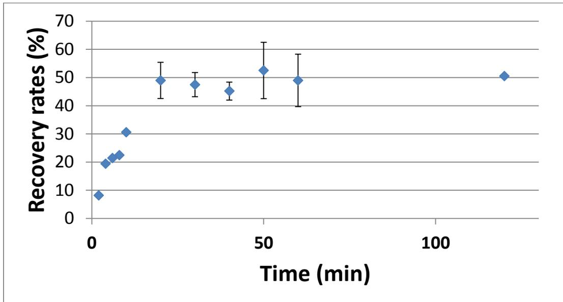
Figure 4: Recovery rates using elution with megasonic assisted agitation
