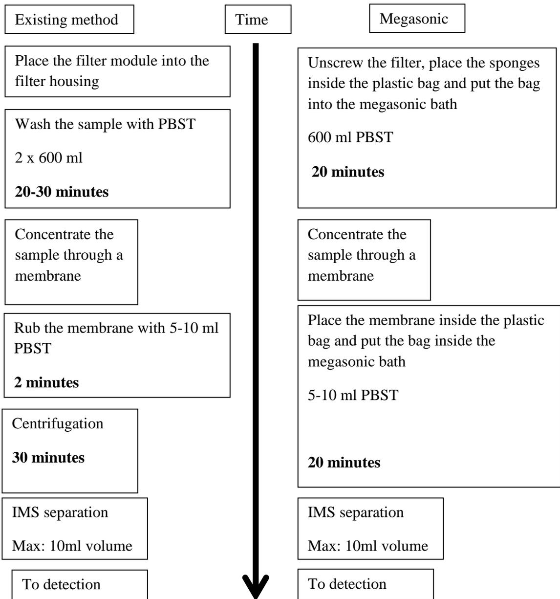
Figure 8: Comparison from a duration point of view between megasonic elution with the existing elution-detection method
