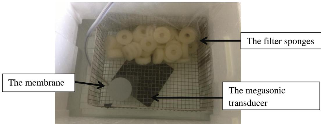
Figure 3: The filter and the membrane inside the Megasonic bath.
