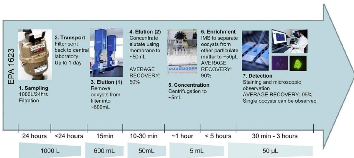
Figure 1: overview of the protocol described in the UK Environment Agency Blue Book publications method for the detection of *Cryptosporidium*. Stage 3 required a minimum of 2 washes of 600 mL. Source adapted from Ref.4
