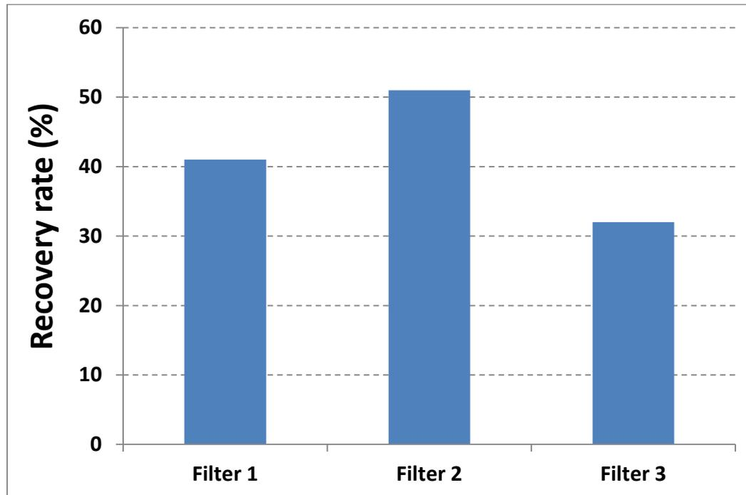
Figure 7: Recovery rates of the three filters (1<sup>st</sup> and 2<sup>nd</sup> stage elution with megasonic)
